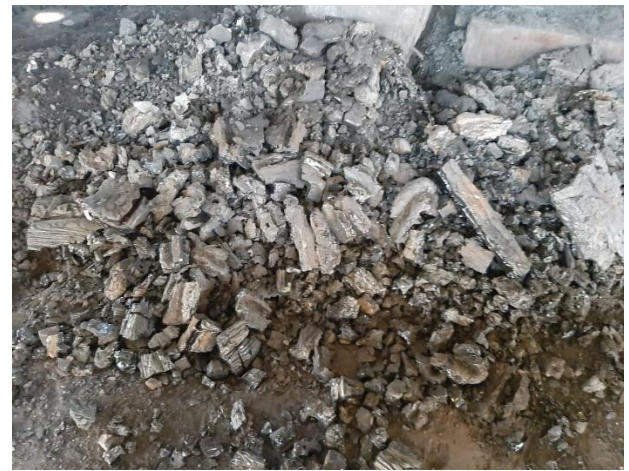
In figure: Slag (waste output from Cupola Furnace which we are using in place of gravels)
